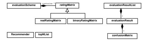
Figure 3: UML class diagram for package **recommenderlab** (Fowler, 2004).
